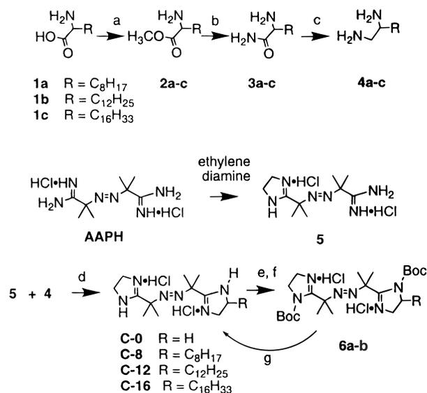
a. MeOH, SOCl<sub>2</sub>. b. MeOH, NH<sub>3</sub>. c. LiAlH<sub>4</sub> d. MeOH, NaOMe, e. NaOMe, f. Na<sub>2</sub>CO<sub>3</sub>/(Boc)<sub>2</sub>O. g. TFAA
